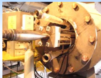
Photo of experimental set up with the discharge chamber and the system to supply O 2 /Ar mixture
